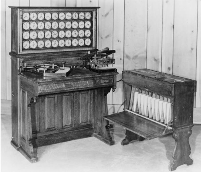
Fig. 30.2 Hollerith's tabulator (1890) (Courtesy of IBM archives)
