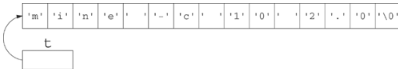
Figure 2.3. The makeargv makes a working copy of the string s in the buffer t to avoid modifying that input parameter.
