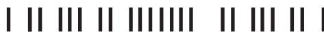
Fig. 2 Example of a complicated anomalous Zeeman splitting (for Runge denominators r_i = 3 and 5 in Runge’s rule, leading to q = 0, \pm 1, \pm 2, \pm 3, \pm 5, \pm 6, \pm 8, \pm 9, \pm 10, \pm 12, \pm 13, \pm 15 ), i.e., 23 components!
