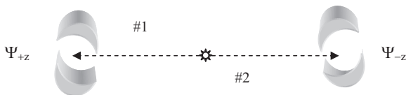
Fig. 1 Two spin-1/2 particles in an entangled state, on which the x -component of spin is measured
