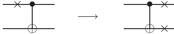
Figure 10.20. A controlled-NOT gate can cause an error to propagate so that instead of affecting one qubit, it affects two. This is also true when encoded qubits are used, and an encoded controlled-NOT is implemented, as discussed in the text.
