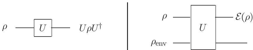
Figure 8.3. Models of closed (left) and open (right) quantum systems. An open quantum system consists of two parts, the principal system and an environment.
