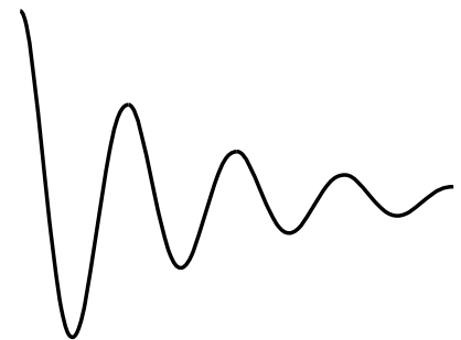
c / The amplitude is halved with each cycle.
