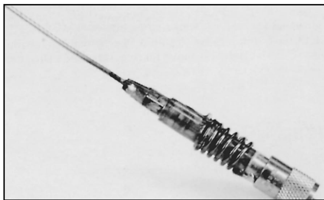
Fig 51 —The 220-MHz 5/8 - \lambda mobile antenna. The coil turns are spaced over a distance of 1 inch, and the bottom end of the coil is soldered to the coax connector.
