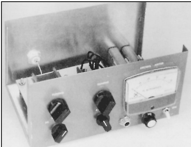
Fig 48 —The linear field-strength meter. The control at the upper left is for C1 and the one to the right for C2. At the lower left is the band switch, and to its right the sensitivity switch. The zero-set control for M1 is located directly below the meter.
