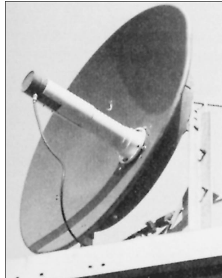
Fig 20— Coffee-can 2304-MHz feed described in text and Fig 19 mounted on a 4-foot dish.
