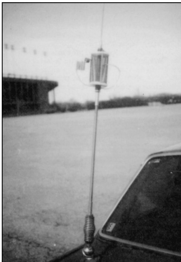
Fig 31—This photo shows the antenna mounted on the trunk of a car. The structure is somewhat cumbersome, so it is guyed appropriately.
