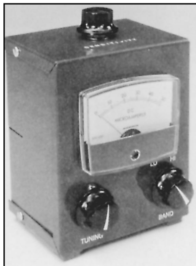
Fig 51 —The RF current probe. The sensitivity control is mounted at the top of the instrument, with the tuning and band switches on the lower portion of the front panel. Frequency calibration of the tuning control was not needed for the intended use of this particular instrument, but marks identifying the various amateur bands would be helpful for general-purpose use. If the unit is provided with a calibrated dial, it can also be used as an absorption wavemeter.
