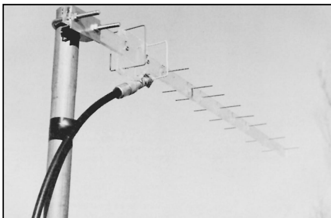
Fig 58 —A view of the 10-element version of the 1296-MHz Quagi. It is mounted on a 30-inch Plexiglas boom with a 3 × 3-inch square of Plexiglas to support the driven element and reflector. Note how the driven element is attached to a standard UG-290 BNC connector. The elements are held in place with silicone sealing compound.
