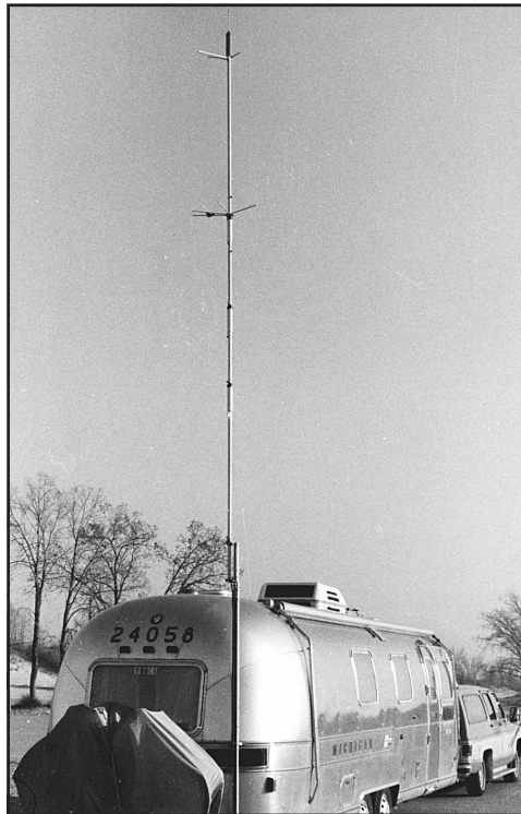
Fig 10 —Ready to go! The W8UCG deluxe RV antenna is shown mounted at the rear of a 31-foot Airstream.
