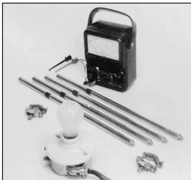
Fig 42—The complete soil conductivity measuring setup. The four probes are cut to 18-inch lengths from an 8-foot copper-coated steel ground rod. (This length provides a measuring stick for spacing the probes when driving them into the soil.) The tip of each probe is ground to a point, and black electricians' tape indicates the depth to which it is to be driven for measurements. Two ground clamps provide for connections to the driven probes.
