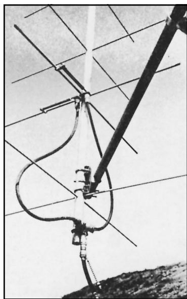
Fig 15 —This VHF crossed Yagi antenna design by KH6IJ was presented in January 1973 QST. Placement of the phasing harness and T connector is shown in the lower half of the photograph. Note that the gamma match is mounted somewhat off element center for better balance of RF voltages on elements.
