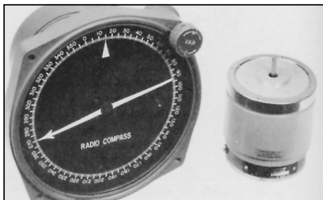
Fig 10 —The MN-98 Canadian radio compass and Sperry R5663642 synchro transmitter. Note the small knob at the upper right-hand corner of the indicator face. This can be used to calibrate the system without making any changes at the antenna end. By turning this knob, you can rotate the degree markings around the outside of the dial face so that any desired heading can be placed in line with the pointer.
