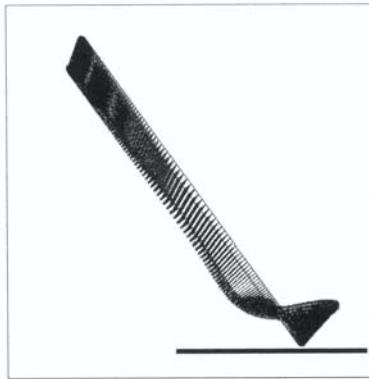
Figure 3. The velocities of the points of the rod after the initial collision with the rigid support. One can note that the rod begins to rotate.
