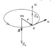
Figure 2. Motion of the centre of charge of the electron around its centre of mass in the C.M. frame.
