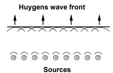
Figure 5. Plane wave formed by Huygens combination of wavelets. The wavelets from a line of sources combine, at a distance from the sources, to form a new wave front which repeats the geometry of the sources.
