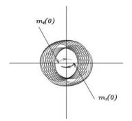
Figure 5: Bound motion of two electrons with parallel spins during a short period of time
