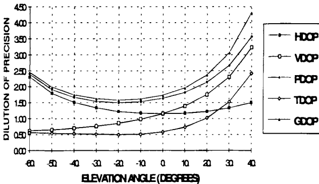
Fig. 1 Dilution of position values for symmetric satellites at various elevation angles above the horizon. The minimum GDOP is at -19.5 deg (i.e., below the local horizontal). This corresponds to locating four transmitters at the apexes of a regular tetrahedron.
