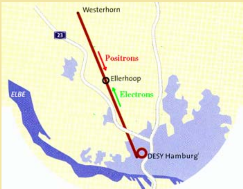
Artist view of TESLA. The machine will have two linear accelerators, each with a length of 15 km. The energy will be 500–800 GeV.
