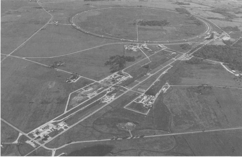
Fig. 19.1. A view from the north of the experimental areas, with the Neutrino Area in the left foreground, the Meson Area to the center right, and the Proton Area in the center left beneath the grove of trees where our buffalo roam. The Main Ring of the accelerator is at the top of this 1977 photograph.
