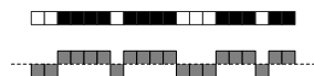
A sequence of discrete elements and a possible corresponding waveform for a sound.
