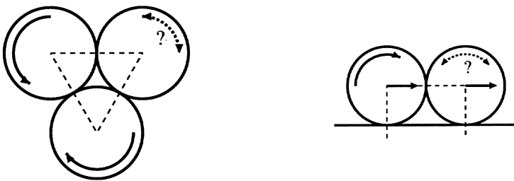
Fig. 12. Frustration of rotational degrees of freedom in the presence of friction
