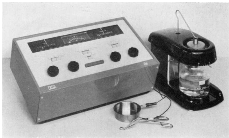
FIG. 1.13. Apparatus for electropolishing specimens. (Courtesy of H. Struers Chemiske Laboratorium.)
