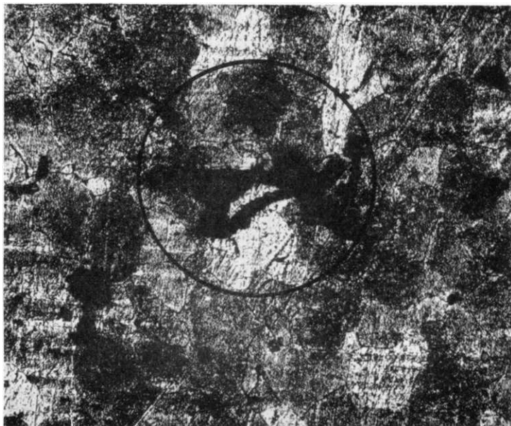
FIG.1.18. (c) Dust adhering to the surface of a specimen.
