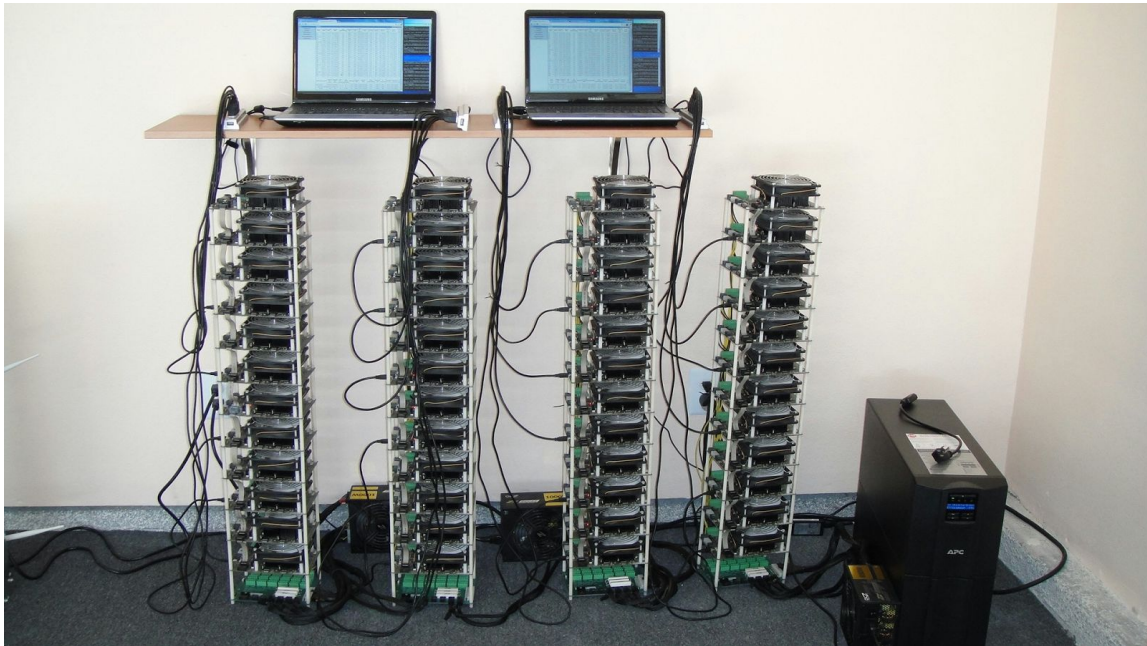
Figure 5.8: A home-built rack of FPGAs. Although you don't see the cooling setup pictured here, a rack like this would need a cooling system.
