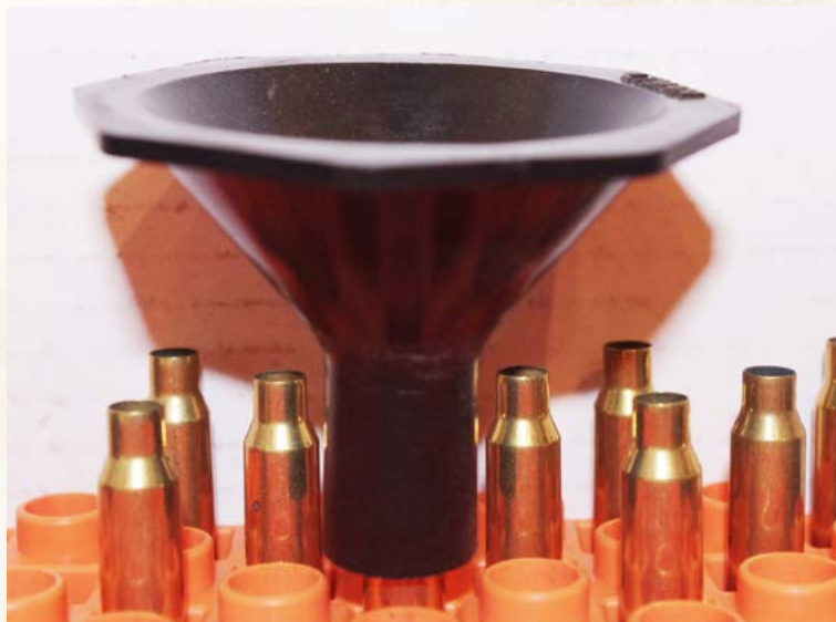
Powder Funnel in Use (Notice how the funnel fits down over the case to prevent spillage)
