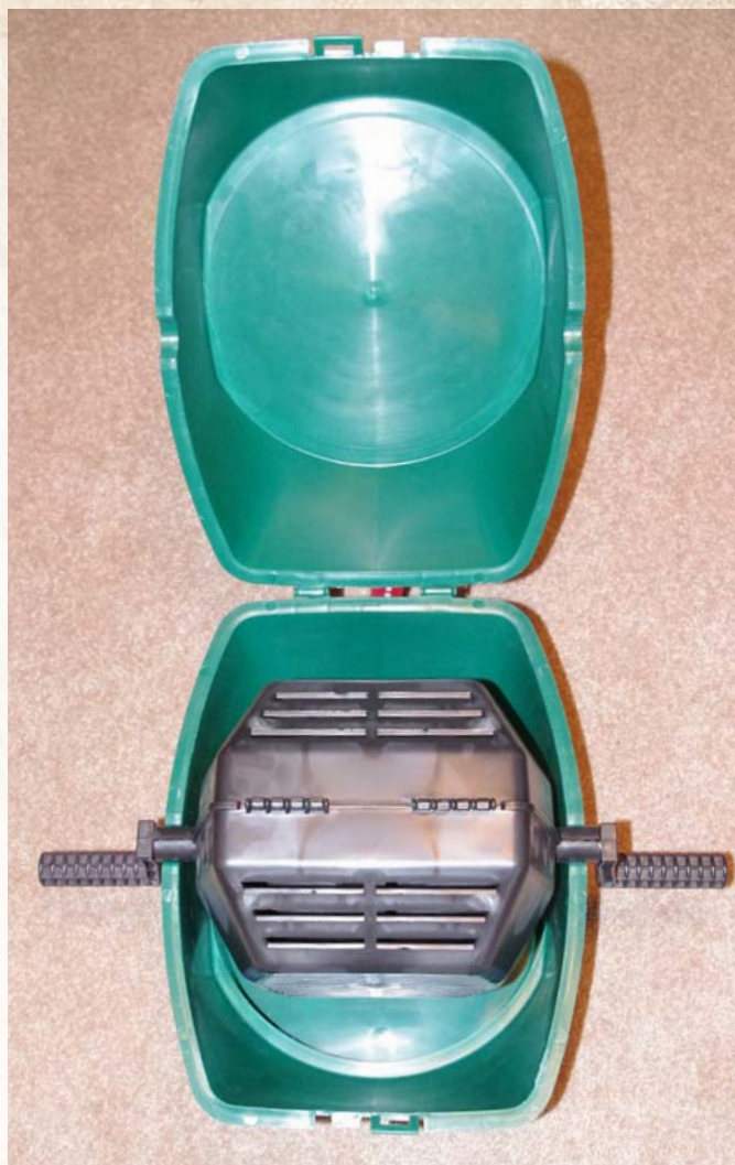
A media separator allows you to quickly separate your cleaned cases from the cleaning/polishing media.
