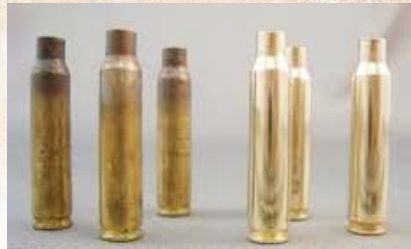
Brass cases before and after cleaning/polishing
