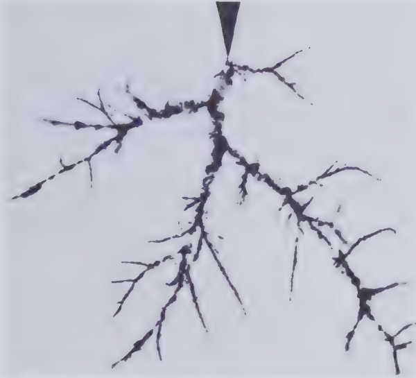
Figure 2.18 Breakdown channels in very viscous hexachlordiphenyl according to Krasucki et al. [2.42]. (Photograph by the Electrical Research Association.)
