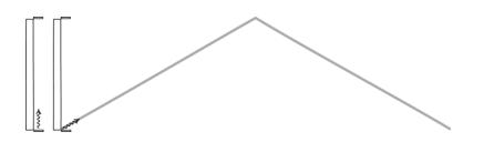
If you watch the animation carefully, you will see that the moving light clock ticks at exactly half the speed of the resting clock. That is because the light signal of the moving clock has to cover twice the distance to go from one end of the rod to the other. To get this doubling of the distance takes a careful adjustment of the speed of the moving clock. It turns out that the moving clock has to be traveling at 86.6% the speed of light.
