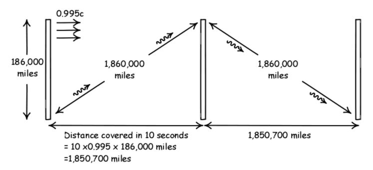
That observer at rest will agree with one that moves with the rod: a light signal leaves one end of the rod and arrives at the other end. But the observer at rest judges that end to be rushing away from the light signal at 99.5% the speed of light. A quick calculation shows that that the signal will now take 10 seconds to reach the other end of the rod.
