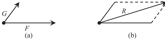
Figure 1. (a) Forces F and G are represented as acting at a single point. (b) Their resultant R is represented by the diagonal of the parallelogram having F 's and G 's representations as adjacent sides.
