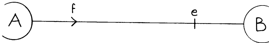
Fig. 3 Interaction bond connecting two system components A and B with dual indices of effort and flow defining the causality of interaction.
