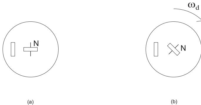
Figure 10.22: The left rectangle represents a wall fixed in the ground. The disc of the gyroscope rotates around its horizontal axis. (a) Initial configuration. (b) Configuration after 3 hours. The gyroscope's axis is precessing relative to the ground.
