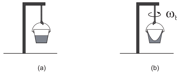
Figure 16.12: Newton's bucket experiment. (a) Bucket and water at rest relative to the ground, with a flat surface of water. (b) Bucket and water spinning together relative to the ground with an angular velocity \omega_b , with a concave surface of water.
