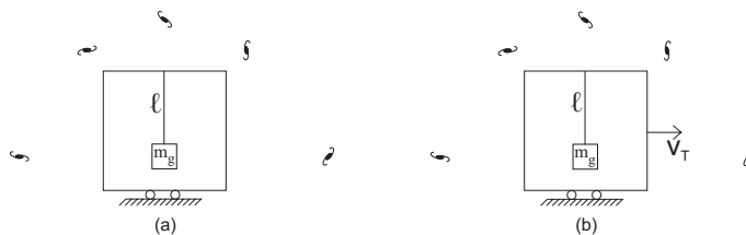
Figure 21.12: (a) Wagon at rest relative to the ground. (b) Wagon, string and test body moving with a constant horizontal velocity v_T relative to the ground.
