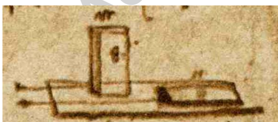
Fig. 5 Sketch showing a block of weight 8 units sliding in two different orientations labelled m and n (CA 198r, c. 1508)
