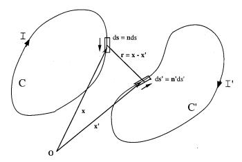
FIG. 1. Two closed current-carrying circuits C and C' with currents I and I', respectively.
