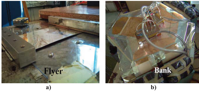
Figure 3 QUATTRO facility for accelerating flyer plates installed at Loughborough University a) Flyer b) QUATTRO bank
